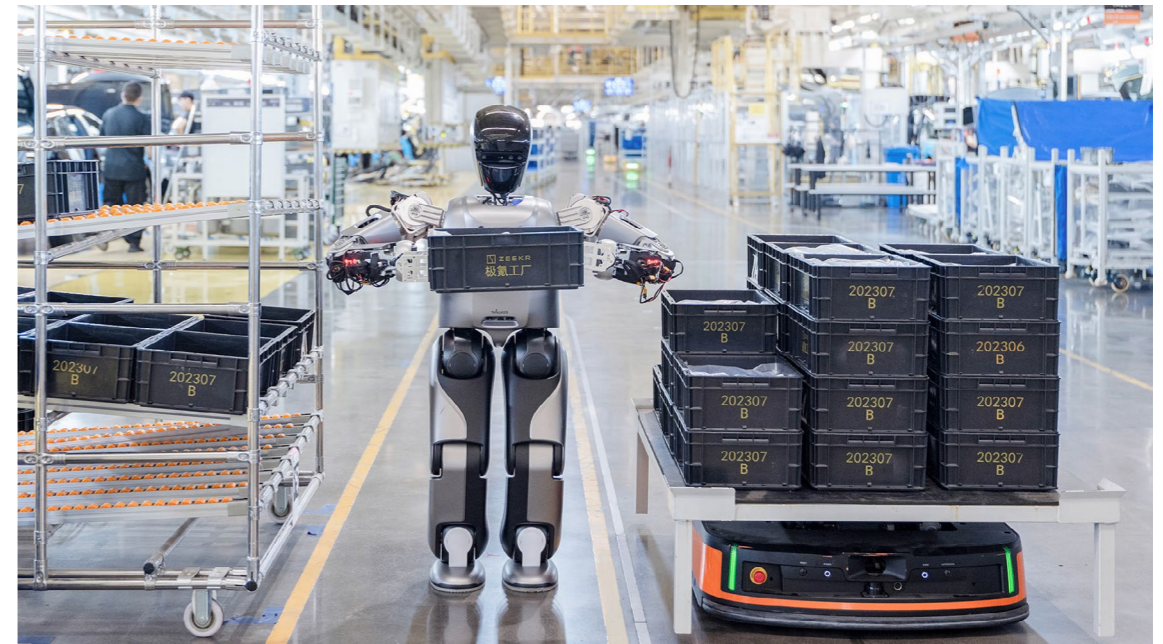
● 优必选工业版人形机器人 Walker S Lite 在极氪 5G 智慧工厂执行搬运任务 ● UBTECH humanoid robot Walker S Lite is working in Zeekr's intelligent factory to complete handling tasks.
