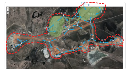
▲ Deployment diagram of phase II of 5G base station in mining area
