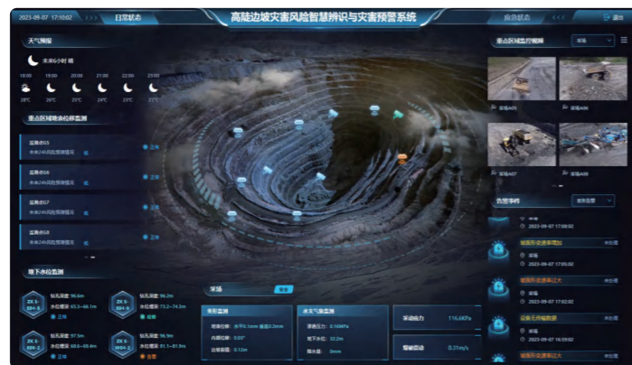
▲ Disaster risk intelligent identification and disaster warning system of high and steep slopes
